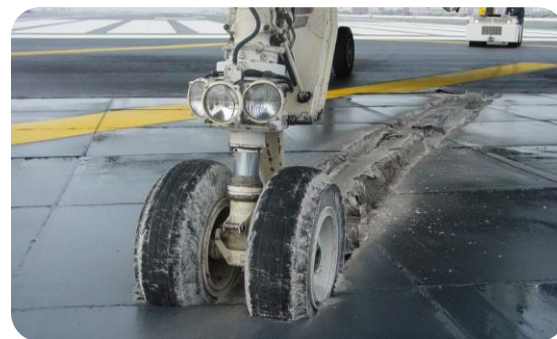
EMASMAX - the premanufactured EMAS block system (runwaysafe.com)
